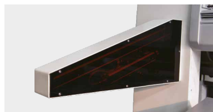
6 Security Photoelectric Protection Device
